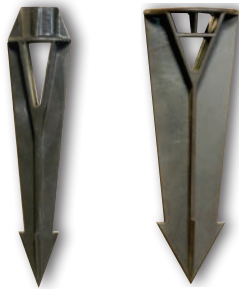
T-193A/T-194A Spikes 1/2" Female NPS Mounting Spikes. T-193A: 2" Dia. x 8 1/2" Long T-194A: 3" Dia. x 8 1/2" Long
