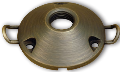
T-190-ERS Cast Brass Mounting Base Shown in Aged Brass (AB) 2 7/8" Dia. x 7/8" High 1/2" NPT Threads
